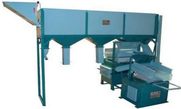
**Seed Destoner Machine:** This machine's aim is to remove stones and other mud material from the given grains.
