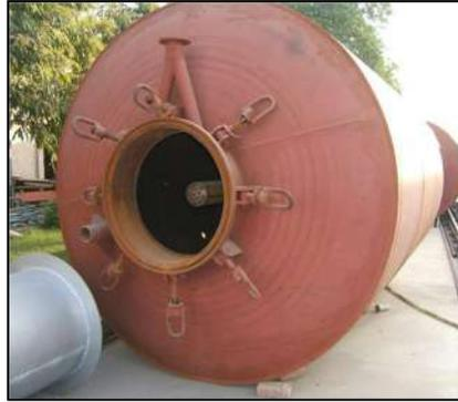
**Fig.:** Pressure Kier System
