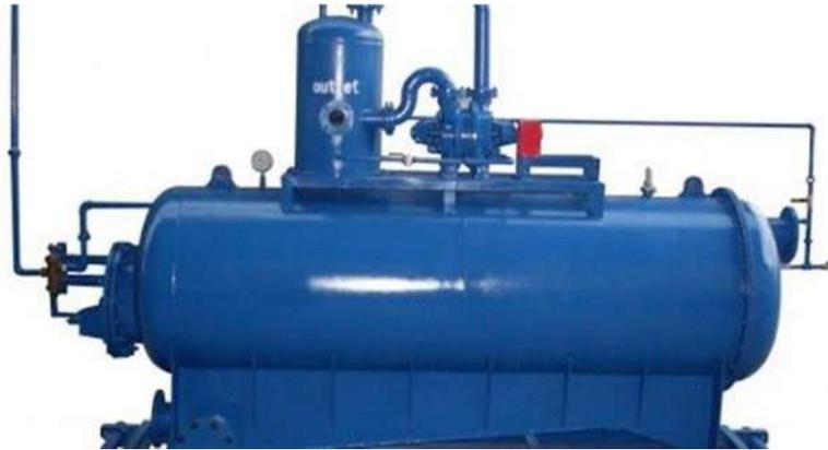
**Fig.:** Vacuum degassing system
