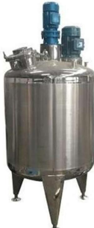
**Fig.:** Jacketed reaction vessel
