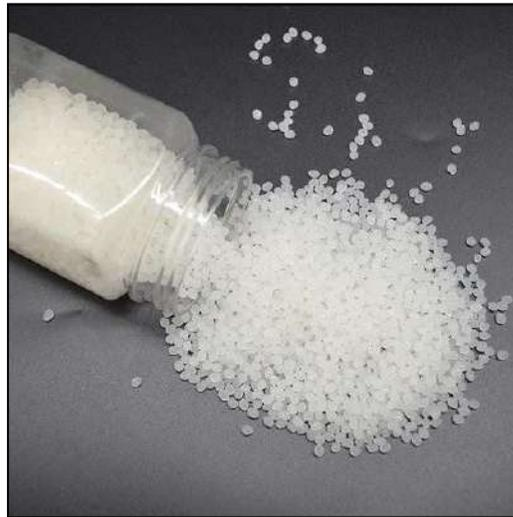
**Fig.:** Biodegradable PLA pellets
