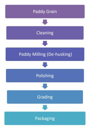
Fig. 1 – Process Flowchart
