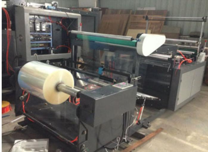
4. **PVC Welding Machine** - This machine is used to weld the bags using profile dies as per the desired dimension.
