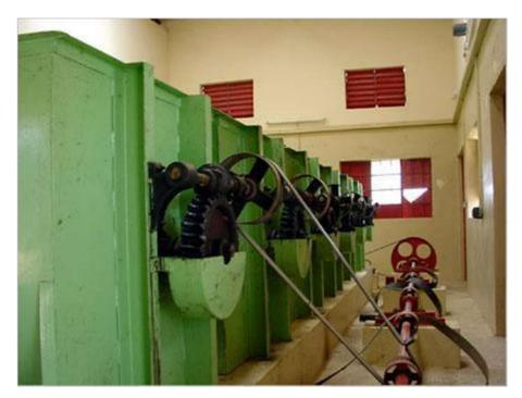
➤ Granulator with Dryer: By being tumbled through heated air in a granulator damp sugar crystals are dried. Vibrating screens are used to sort the dry sugar crystals by size and put them into storage containers.
