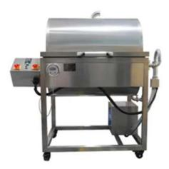
✓ **Honey Mixing Machine:** The dehydrated honey channelized into the mixing chamber where solvent is mixed to upgrade its quality.
