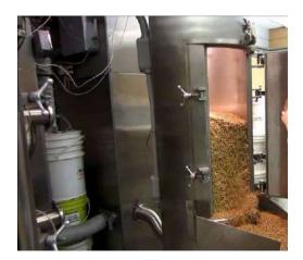
➤ Lauter Tun- The Lauter Tun is a vessel used to separate the wort from the mash solids. It usually has a false bottom with a slotted, perforated floor that retains the spent milled grains while enabling the wort to filter through the grain bed and gather in the area beneath; the wort then flows to the brew kettle.
