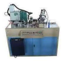
> Arc welding machine: This machine is use to form continues weld on the electric horn.
