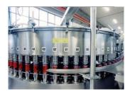
This equipment is used to fill the finished product in cans of different sizes.
