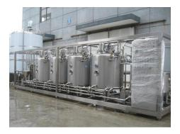
This equipment is used to heat and thus evaporate the water from milk in a controlled manner.
