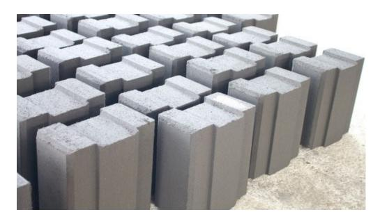
**Shapes & sizes:** A variety of interlocking blocks have been developed during the past years, differing in shapes and sizes, depending on the required strengths and uses. The system developed has the following shapes and forms:
