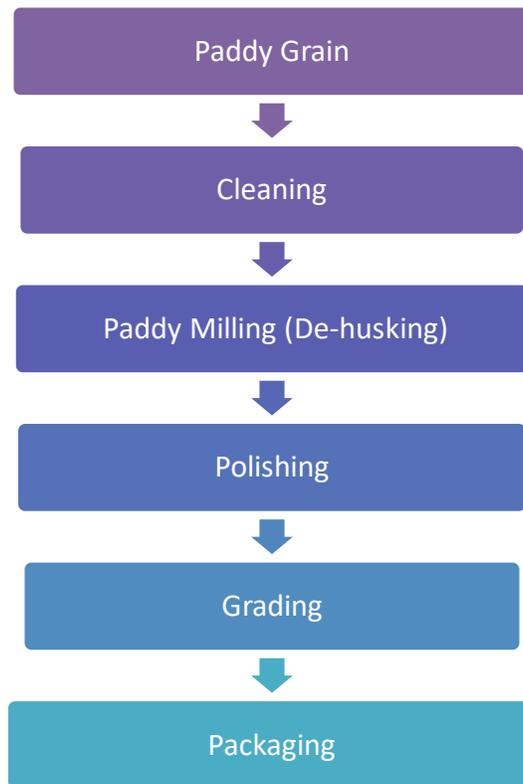
Fig. 1 – Process Flowchart
