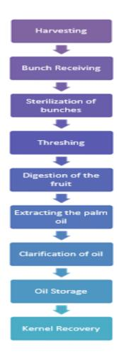
Fig. 1 – Process Flowchart
