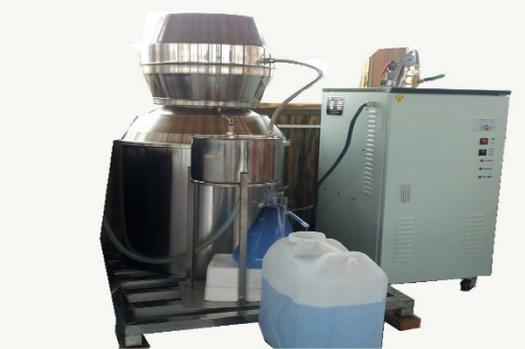
An industrial electric distillation unit consisting of a large stainless steel boiler with a hemispherical top, connected to a condenser and a collection vessel. A control panel with various gauges and switches is visible on the right side.                |
