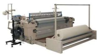
Loom is a fabric manufacturing machine which is used to weave a fabric, the air jet loom utilizes air jets to insert the weft to form the woven fabric.
