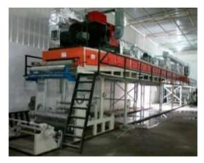
The machine has a roll unwinding station, tape alignment and tensioning station, coating station, drying station, roll winding station and tape slitting station; these stations are in general required for any adhesive tape manufacturing.
