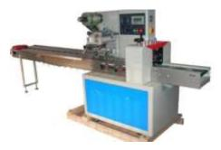
This machine simply packs the adhesive plaster within a plastic packaging.
