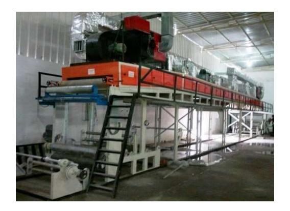
The machine has a roll unwinding station, tape alignment and tensioning station, coating station, drying station, roll winding station and tape slitting station; these stations are in general required for any adhesive tape manufacturing.
