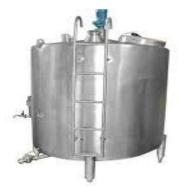
In dairy and milk processing industry a bulk milk storage tank is a large storage tank for holding the milk at a cold temperature until it can be picked up by a milk hauler. It is made up of stainless steel and is used every day to store the raw milk on the farm in good condition.
