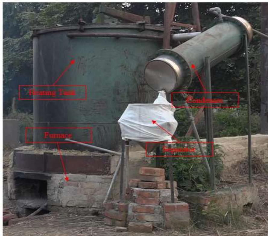
Field Distillation Apparatus
