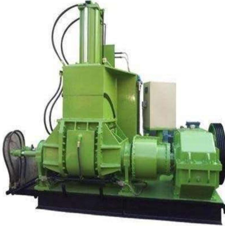
3.2.4 Mixer with Heating Arrangement- It is a combined machine used to mix the components along with heating the mixed substance.
