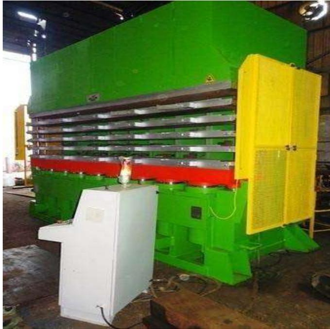
3.2.9 Tube Curing Machine-Curing is a process that involves a chemical reaction (polymerization) or a physical action (evaporation) that produces a stronger, tougher, or more stable linkage (such as an adhesive connection) or material (such as concrete).
