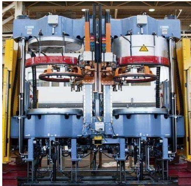
3.2.8 Pre-cured Tread Machine-The "Pre-cured Tread Rubber Retreading Process," also known as "Cold Process Retreading," is a new technology that has been created. This technique eliminates the requirement for a tread matrix at the vulcanizing step since the Pre-cured Tread Rubber already has a tread pattern on it.
