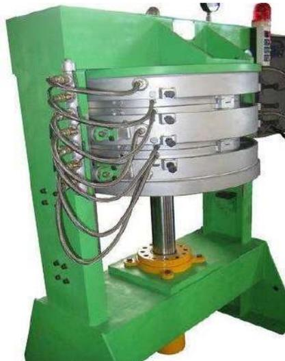
3.2.10 Tube Joining Machine-Pipe joints are connectors at the ends of pipe sections that allow two pipe sections to be connected together to form a pipeline of any length.
