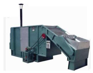
➤ **Grading Machine:** Tea grader is a technical machine helps to identify the defects of buds according to size, shape, and color.
