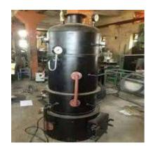
Steam distillation unit-utilized to effectively extract one or more components of a solution or mixture.
